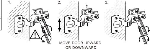
Unscrew 2 screws in round holes loosen 2 screws in oval holes a bit. Tighten 2 screws in oval holes. Screw in 2 screws in round holes
